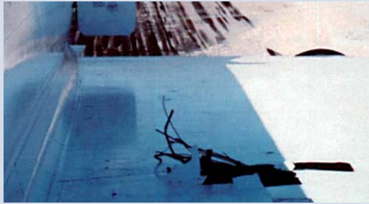
Air France Concorde flight 101 on the 14 th of June 1979, that blew two tyres on the left hand main gear while taking off from Washington which caused perforation of the fuel tank, all the way through the wing. The gear could not be retracted, so the crew elected to return to Washington. Some circuitry was damaged after having been hit by debris from the tires. Debris also caused a fuel and hydraulic leak.
